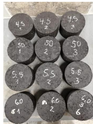
Figure 4. Briquettes used in the Marshall Test.
