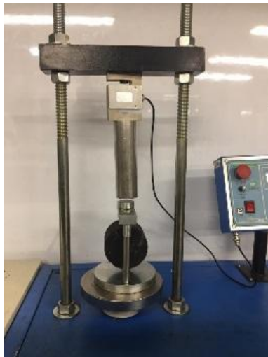
Figure 5. Indirect tensile strength test.
